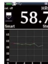
Smart display mode, can set tolerance, automatically reject the result when out of tolerance
