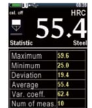
Statistics display mode, show maximum, minimum, deviation, average, relative range and test times
