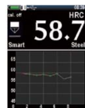
Smart display mode, can set tolerance, automatically reject the result when out of tolerance
