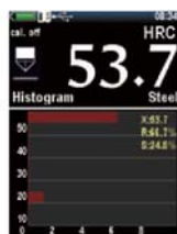
Histogram display mode, show average value, relative range and relative standard deviation
