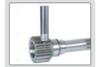
ultrasonic probe to test narrow areas (remove the cover)
