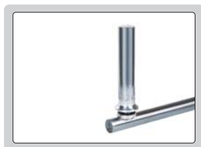
test cylinder surfaces (use V-groove on the cover)
