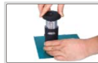
step 3: rotate the handwheel, read the adhesion when dolly is pulled off
