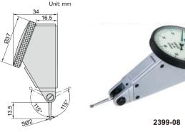
Code **Dial Reading** Range Graduation **Accuracy** Hysteresis 2399-08\* 0.8mm 0-40-0 0.01mm 13µm 3µm
